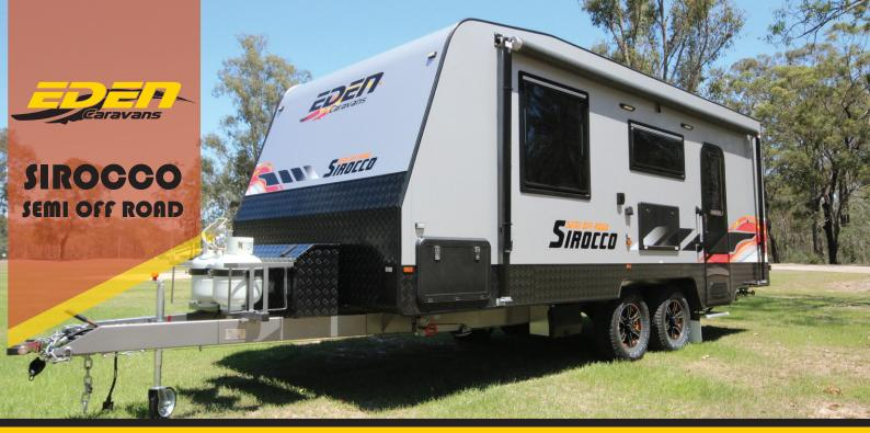
20ft Van (With tunnel boot) - Tare Mass: 2360kg - Ball: 120kg - ATM: 2860kg
